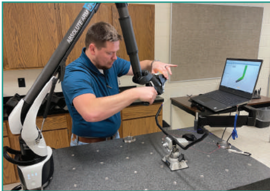
Project Engineer using RS6 Hexagon 3D Scanner
