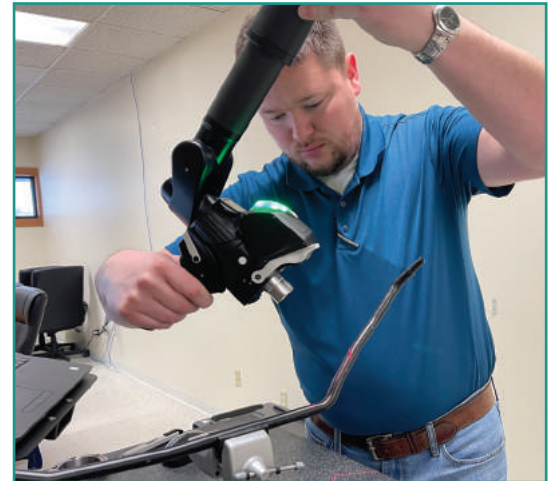
Project Engineer using RS6 Hexagon 3D Scanner
